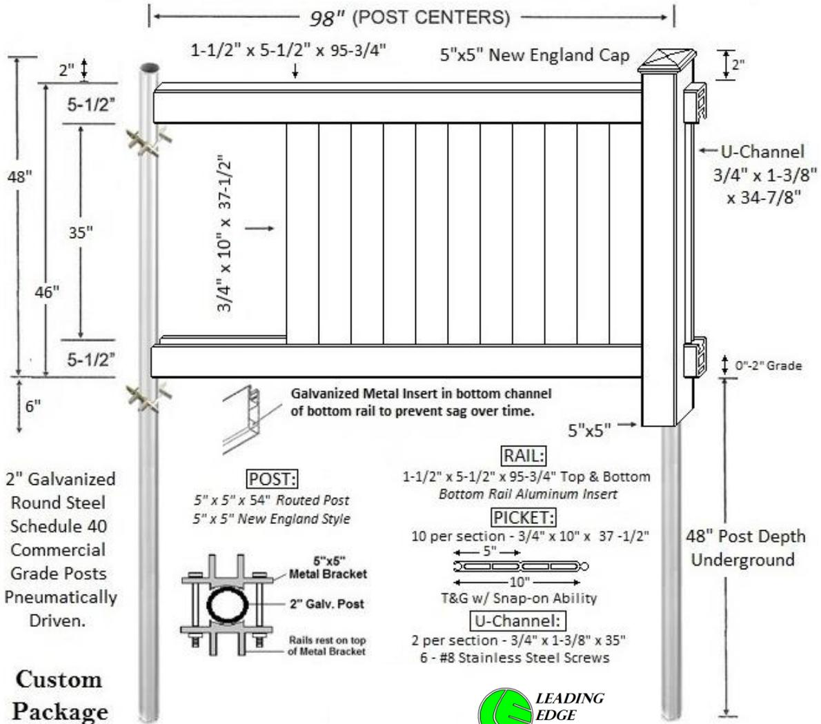
2" Galvanized Round Steel Schedule 40 Commercial Grade Posts Pneumatically Driven.
