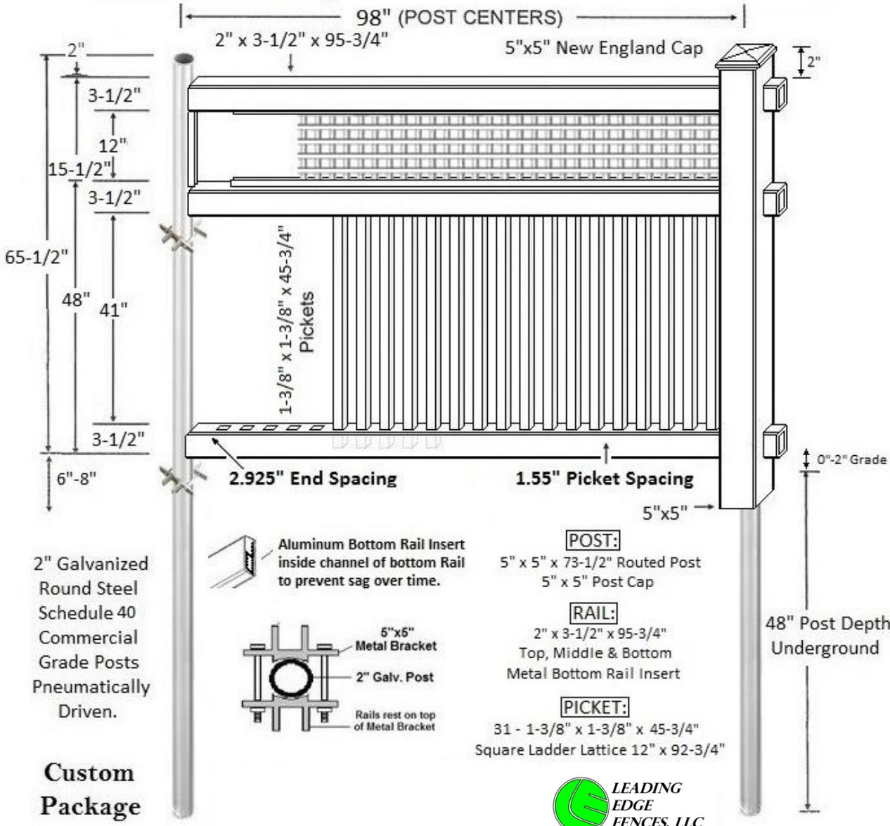
2" Galvanized Round Steel Schedule 40 Commercial Grade Posts Pneumatically Driven.
