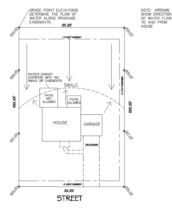
Diagram B: Example of the slopes and swales that may be present on a carriage lane / alley home.
